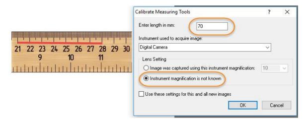
Note: the longer the line the more accurate the calibration.
